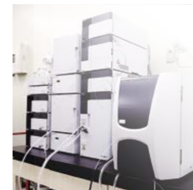
Measurement of the molecular size distribution of dissolved organic matter (DOM) Size exclusion chromatography system with a total organic carbon (TOC) detector
