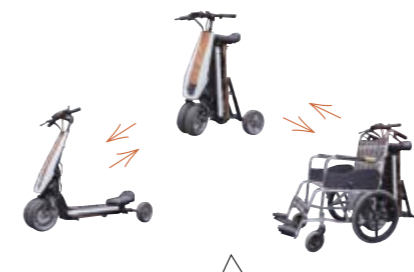
The ultra-compact personal mobility system can be transformed to suit the user type and the purpose of use (multi-purpose mobility).
