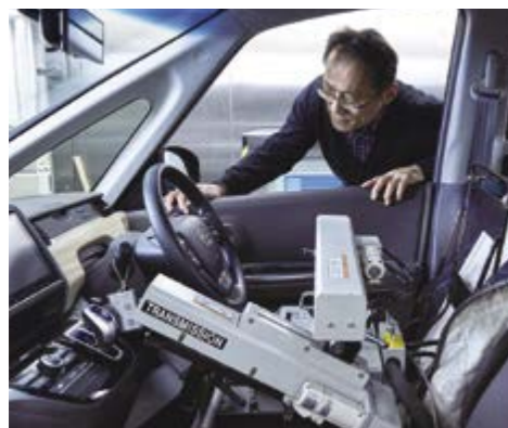
Automated driver (robot) instead of a human driver
