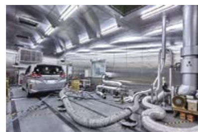
Vehicle on a chassis dynamometer in the environment simulation room
