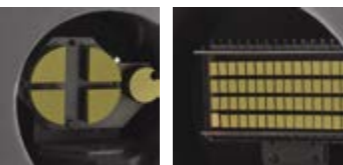
Multi-reflection mirror for infrared spectroscopy
